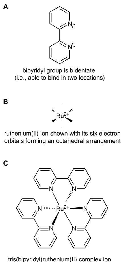
Figure 2. Structures of (A) bipyridyl group, (B) ruthenium ion showing octahedral symmetry, and (C) tris(bipyridyl)ruthenium(II) ion.
