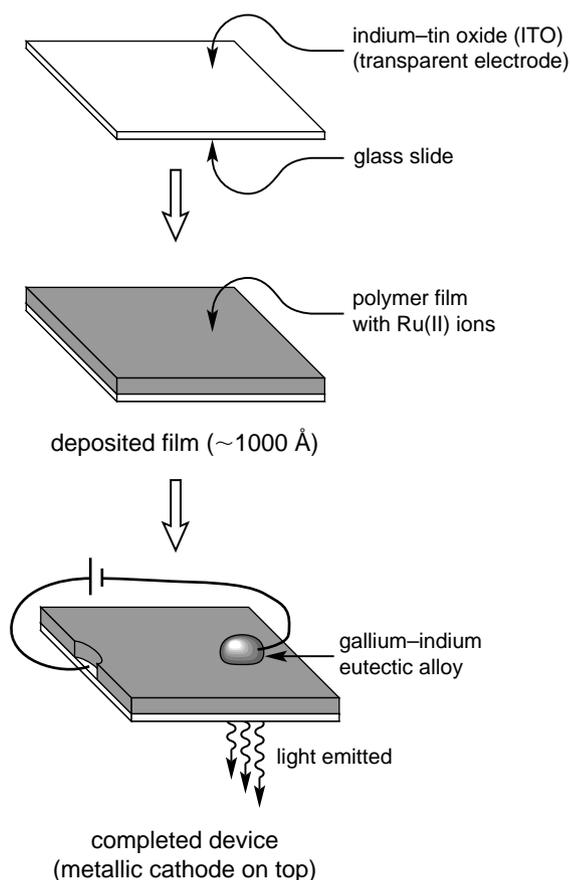
Figure 1. Device fabrication: Begin with glass slide coated with ITO. Spin-coat thin film containing  $[\text{Ru}(\text{bpy})_3]^{2+}$  and  $\text{Cl}^-$  ions embedded in polymer matrix. Place metallic Ga–In cathode on top of thin film and connect Ga–In and ITO to voltage source to emit light.
